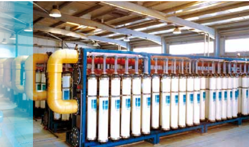
50,000 m 3 /day seawater membrane filtration system
